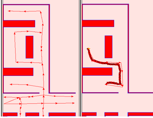
Fig. 4. The figure's left side shows the topological map of the environment, the right side shows the path generated by a potential fields approach combined with the Dijkstra algorithm
