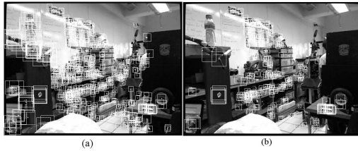
Fig. 3. Neighborhoods computed by (a) FAST and (b) FAST+3D. Notice how many regions that are less likely to be repeatable at different viewpoints (real object corners and edges) are removed by FAST+3D.
