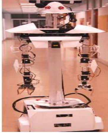
Fig. 2: Robot Justina with one Kinect device in the top of its mechatronic head.
