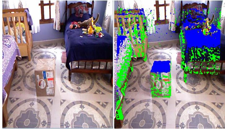
Fig. 1: 3D scanning of a room, the left side shows a picture of the room to be scanned, the right side shows the horizontal and vertical planes of it, found using the 3D cloud points obtained by a Kinect device.
